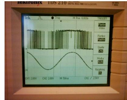
The two low pass filter forms a well suited sine wave out of the pwm signal. The first works as an integrator, the second eliminates the rest of the pwm signal which are still on the sine wave.
