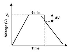
Where  $R_d$  is the ESR<sub>DC</sub> in Ohms  $\Delta V$  is the voltage drop after 10mS I= discharge current
