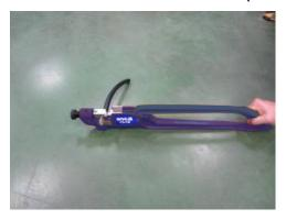
7. Open the handle and check the if the terminal and cable crimped properly..
