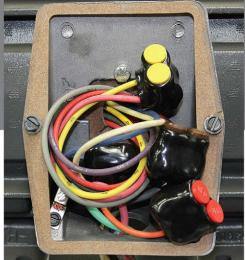
NIMBUS4FLEX Motors are available to order as single catalog numbers, Type PBTI, or as preconfigured kits, Type PBTFML, for specific motor applications. These products provide a superior connection to traditional installation methods such as twist-on wire caps and split bolts with tape.
