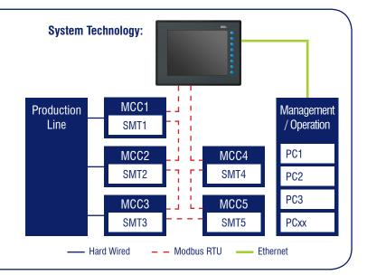
To improve productivity the client wished to monitor OEE of the existing grain processing and cleaning line. Although retrofitting of the data collection points would require modifications in several control panels, it would be necessary to keep production disruption to a minimum.
