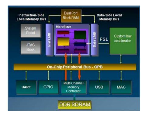
In this example, a software application running on the MicroBlaze communicates with the hardware FIR filter using Impulse C API functions/macros, which are implemented by the Impulse C compiler using FSL.
