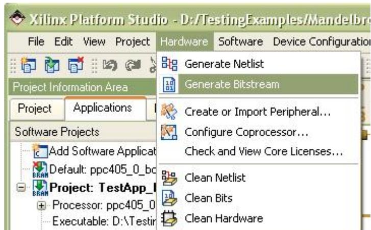
After the bitstream generation has completed, make sure your **JTAG** cable is plugged in properly and the **ML403** board is powered up. Select **Download Bitstream** from the **Device Configuration** menu as shown below:
