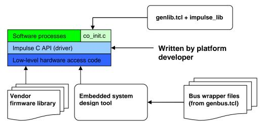
Figure 24: Implementing Impulse C software drivers
