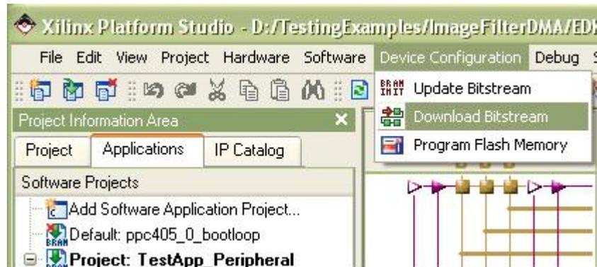
When the FPGA has been successfully programmed, you will see a "Programming Complete" message in the Platform Studio transcript, and you will see a small row of LEDs located light up in sequence on the lower right corner of board.
