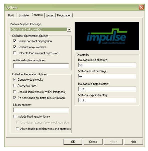
Specify Xilinx Virtex-5 APU (VHDL) as the Platform Support Package. Also specify hw and sw for the hardware and software directories as shown, and specify EDK for both the hardware and software export directories. Also ensure that the **Generate dual clocks** option is checked, which will allow the
