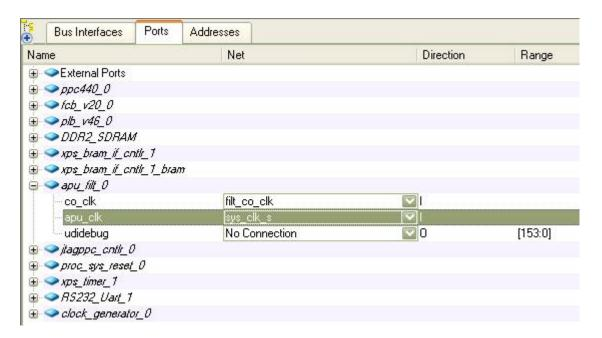
Note: if **co\_clk** is missing from the **apu\_filt\_0** section, then will need to return to <u>step 3</u> of this tutorial and specify the **Dual Clock** option in the **CoDeveloper Generate Options** page.
