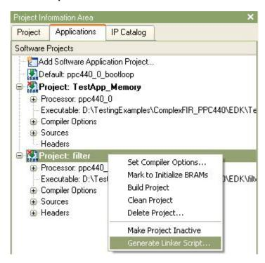
The **Generate Linker Script** dialog will appear. Make sure that all the sections in the **Sections View** are using **DDR2\_SDRAM** as memory. For the **Heap and Stack**, enlarge the size to **0x1000 bytes**, and also use **DDR2\_SDRAM** as memory.
