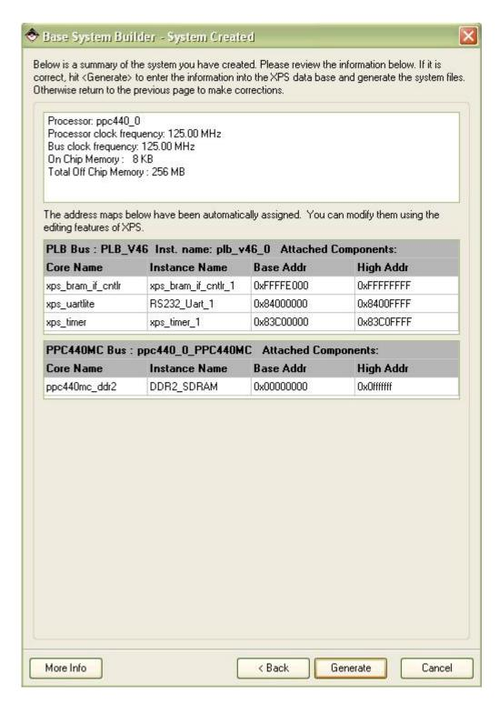
Click **Generate** to generate the system and project files. After this is done, the **Base System Builder** will display the **Finish** page as shown below:
