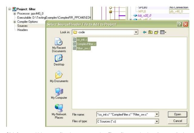
Click **Open** to add the source files shown to your project. These files comprise the software application that will run on the PowerPC CPU.
