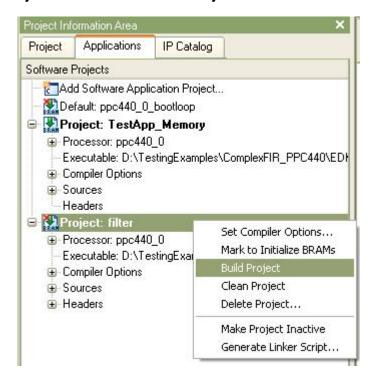
The on-chip memory is not enough for the project. The instruction and data sessions need to be put into external **DDR2 SDRAM**, and also for the heap and stack. To do this, right-click the **Project: filter**, and select **Generate Linker Script...**
