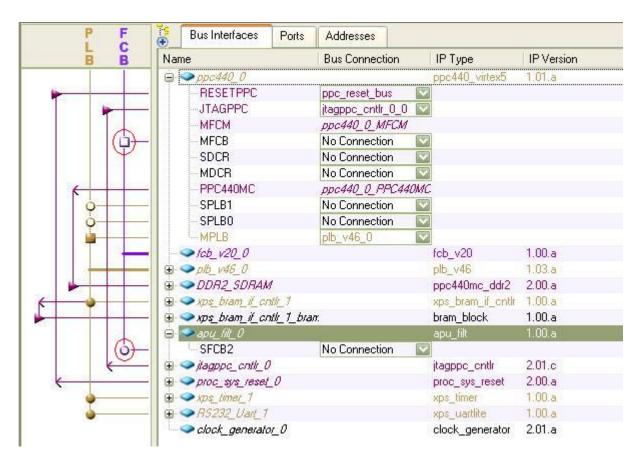
Notice that there are an empty square and an empty circle on the **FCB** bus. Click the empty square to connect the **ppc440\_0**'s **MFCB** interface to the **fcb\_v20\_0** bus. Click the empty circle to connect the **apu\_filt\_0**'s **SFCB2** interface to the **fcb\_v20\_0** bus. They should be connected as shown below:
