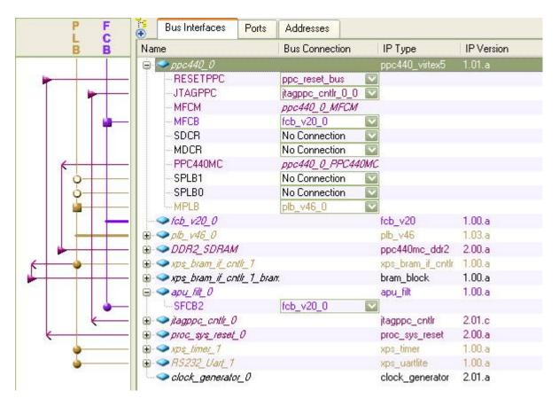
Two ports have to configured for the FCB. Click on the Ports tab in the System Assembly View and expand fcb\_v20\_0 IP core. Set SYS\_Rst to sys\_bus\_reset and set FCB\_Clk to sys\_clk\_s as shown.
