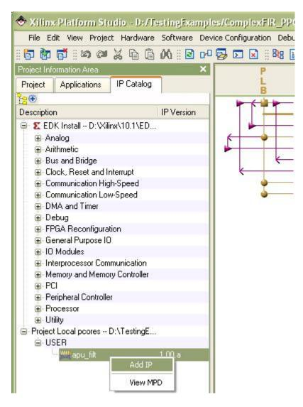
The apu\_filt module will appear in the list of peripherals in the System Assembly View on the right.
