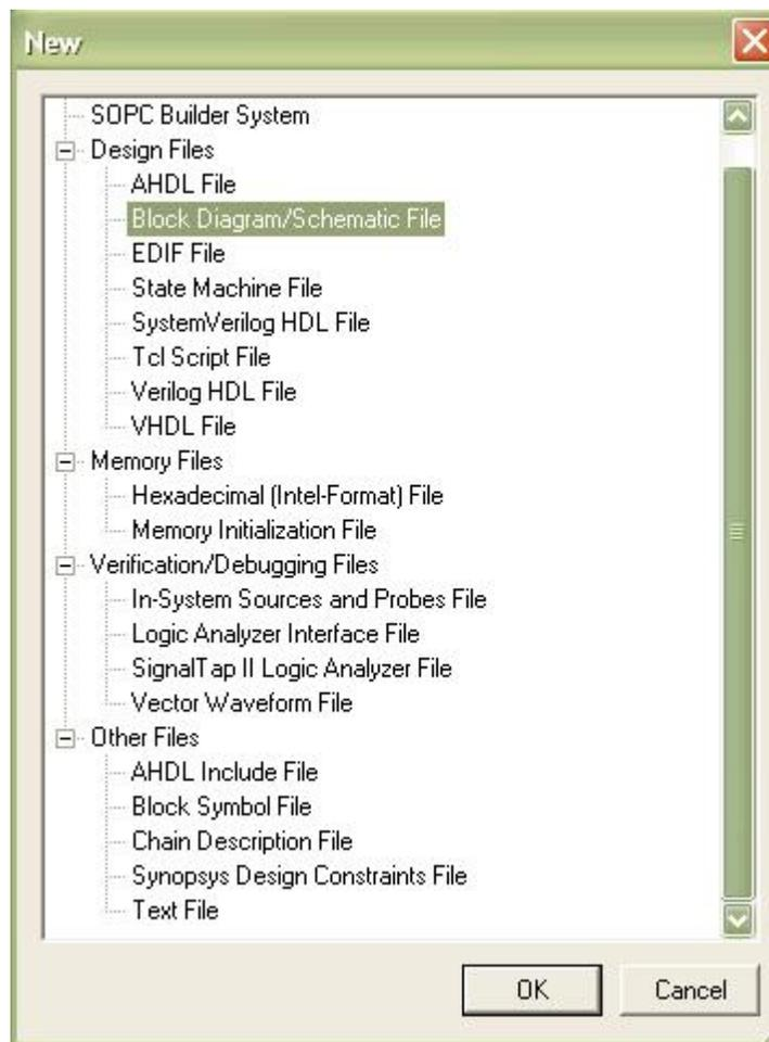
Click OK, and a new DBF file will appear. Now add the block representing the SOPC Builder-generated system. Double-click anywhere in the new block diagram file to bring up the **Symbol** dialog. Open the **Project** folder and select the **HelloWorldSystem** symbol as shown below:
