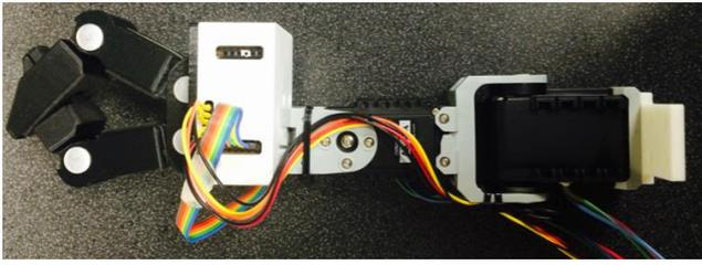
Fig. 4. Snapshot of the first prototype of the Astrobee perching arm.
