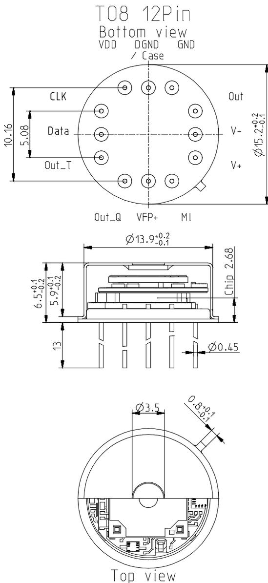
Maximum current between Case and the "Case"-Pin 10 mA!
