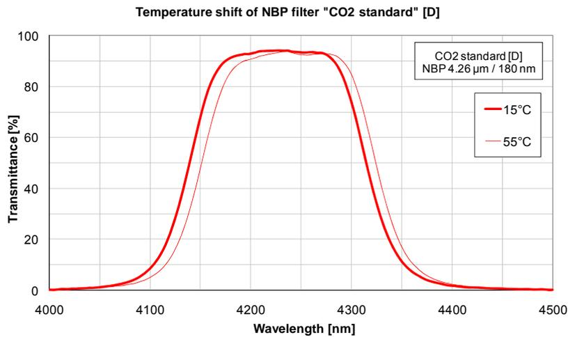
Fig 3: Temperature shift of NBP filter with low TC design
