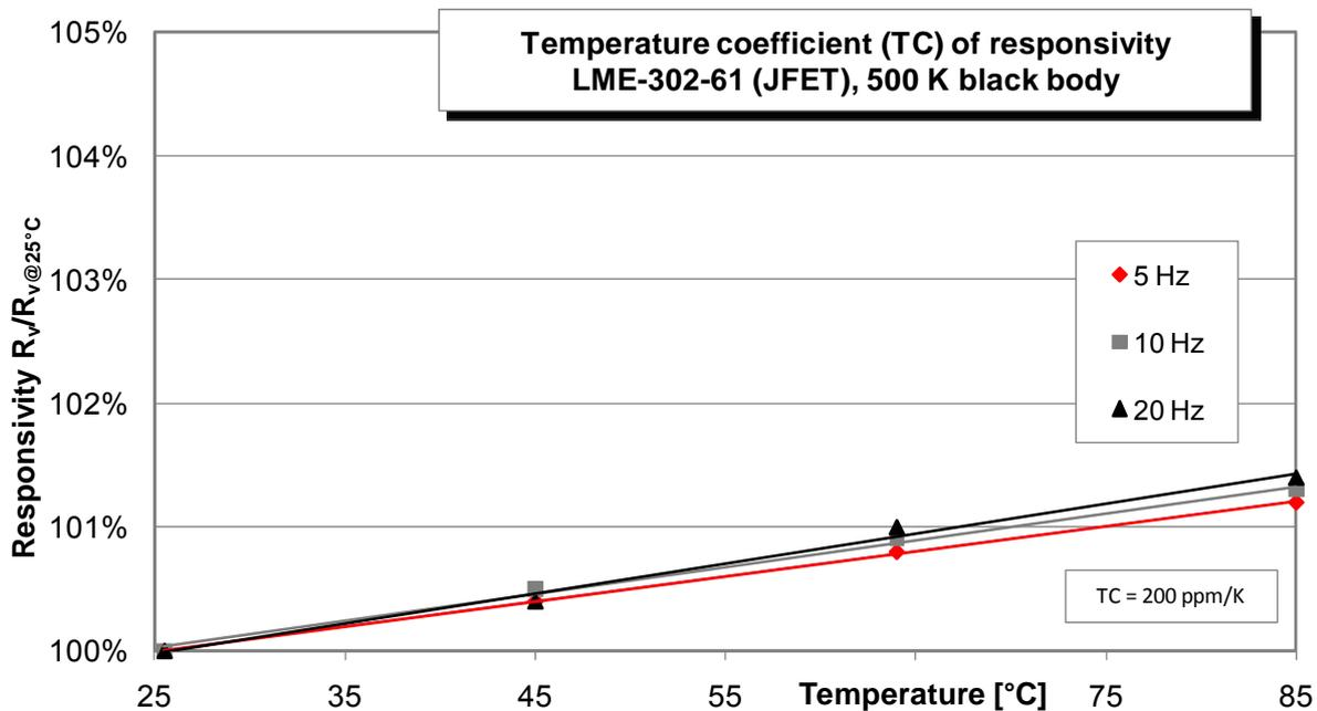
Fig 5: LME-302-61 (single channel; TO39 housing; medium chip size; low Micro; JFET; voltage mode; ch1: CaF2 0.7 mm thick)
