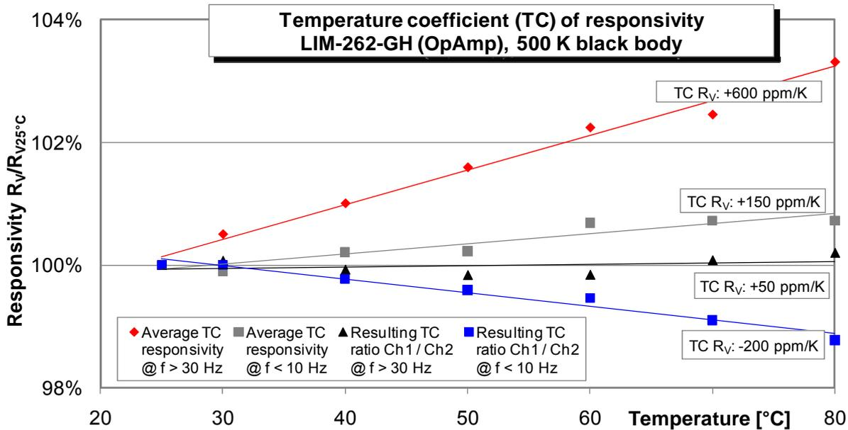
Fig 8: Dual channel detector LIM-262-GH (TO39 housing; small chip size; thermal compensation; OpAmp; current mode; feedback 100 GOhm; ch1: NBP 3.40  $\mu\text{m}/120\text{ nm HC}$ ; ch2: NBP 3.95  $\mu\text{m}/90\text{ nm Ref}$ ), identical filter placement as with the LIM-222-GH in figure 7.
