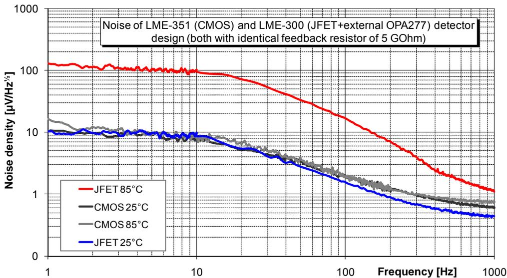
Fig 2: Different behavior of JFET and CMOS input transimpedance amplifiers at temperature increase
