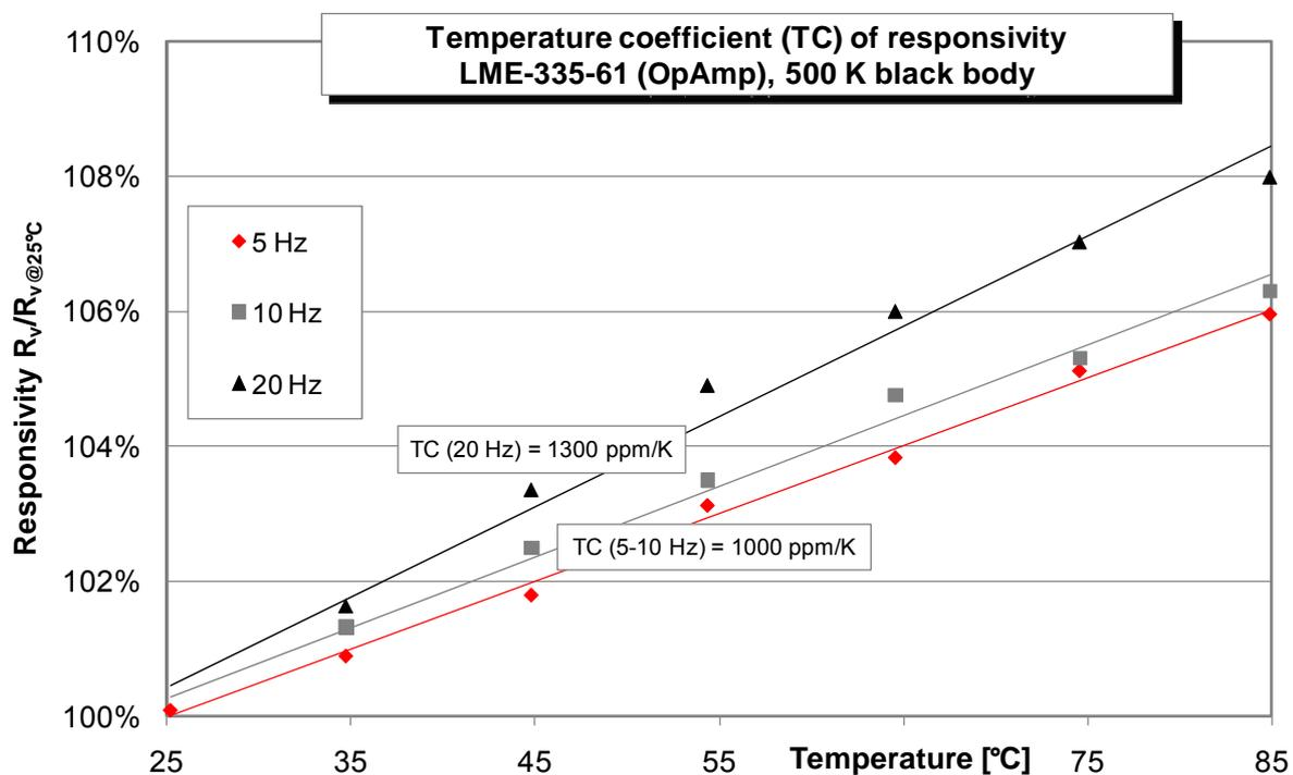
Fig 6: LME-335-61 (single channel; TO39 housing; medium chip size; thermal compensation; low Micro; OpAmp; current mode; feedback 100 GOhm; ch1: CaF2 0.7 mm thick)
