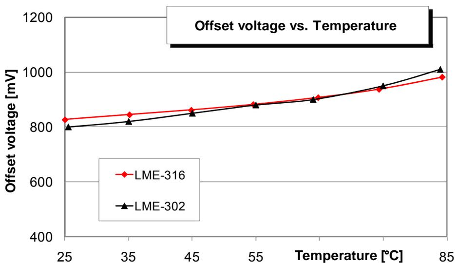
Fig 9: Offset voltage vs. temperature (JFET circuitry); after thermal transient period
