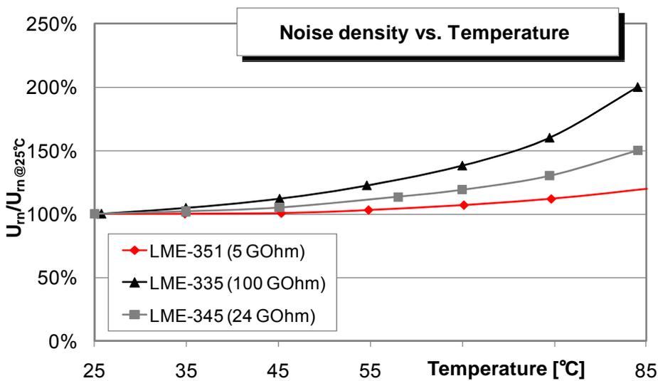
Fig 12: Noise density vs. temperature (current mode detectors with OpAmp)
