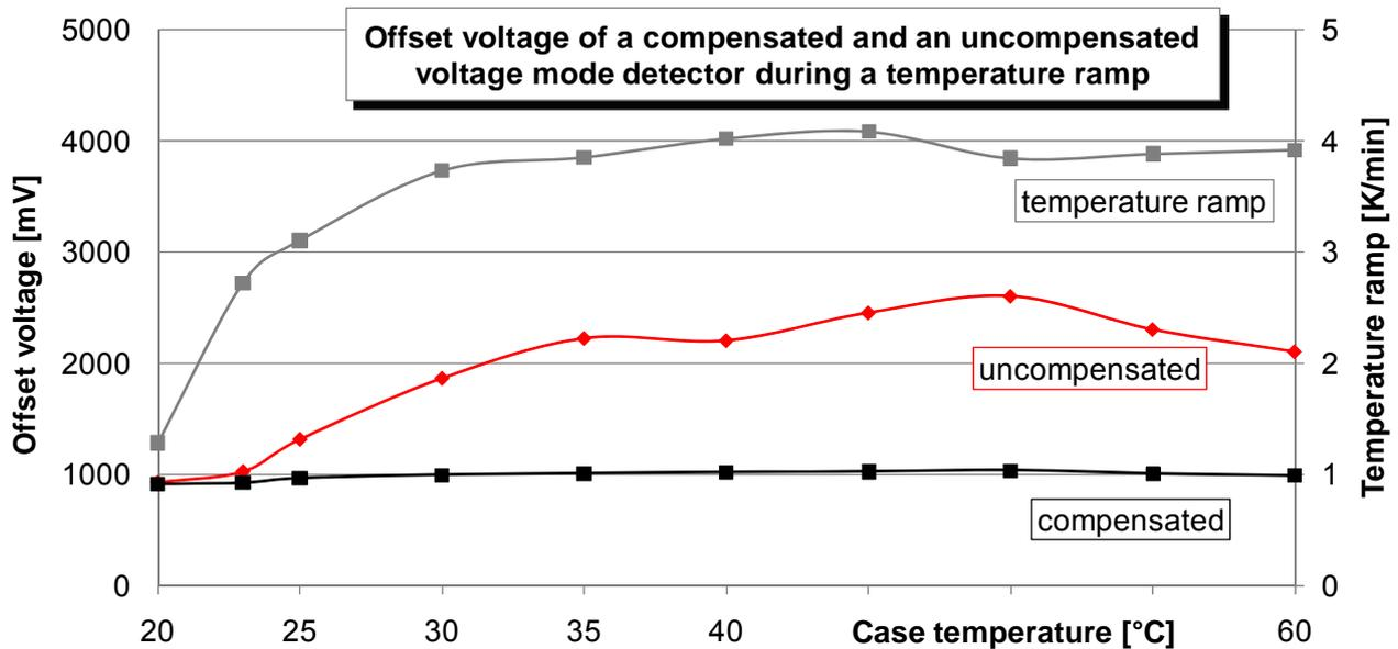
Fig 14: Offset voltage vs. temperature (compensated and uncompensated voltage mode detectors, JFET circuitry)
