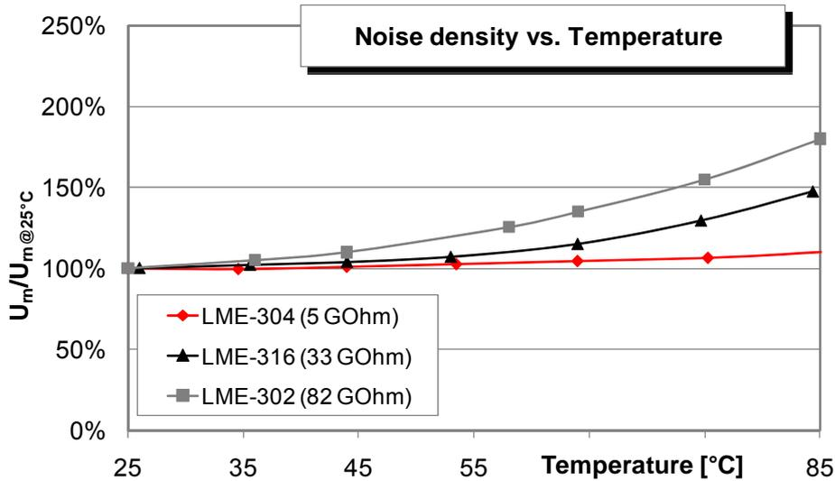
Fig 11: Noise density vs. temperature (voltage mode detectors with JFET)
