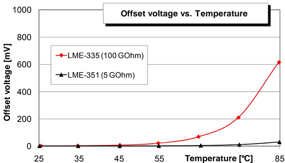
Fig 10: Offset voltage vs. temperature (OpAmp circuitry); after thermal transient period
