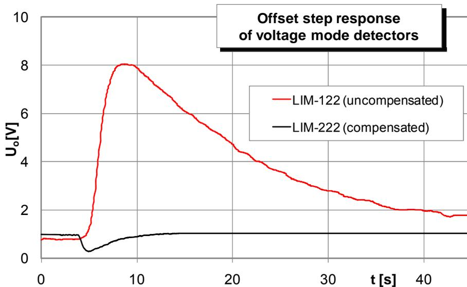
Fig 16: Change of offset voltage vs. time of typical voltage mode detectors after fast temperature increase
