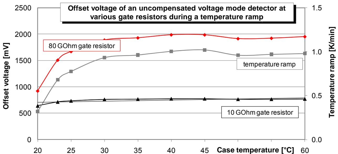
Fig 13: Offset voltage vs. temperature at various gate resistors (uncompensated voltage mode detector, JFET circuitry)
