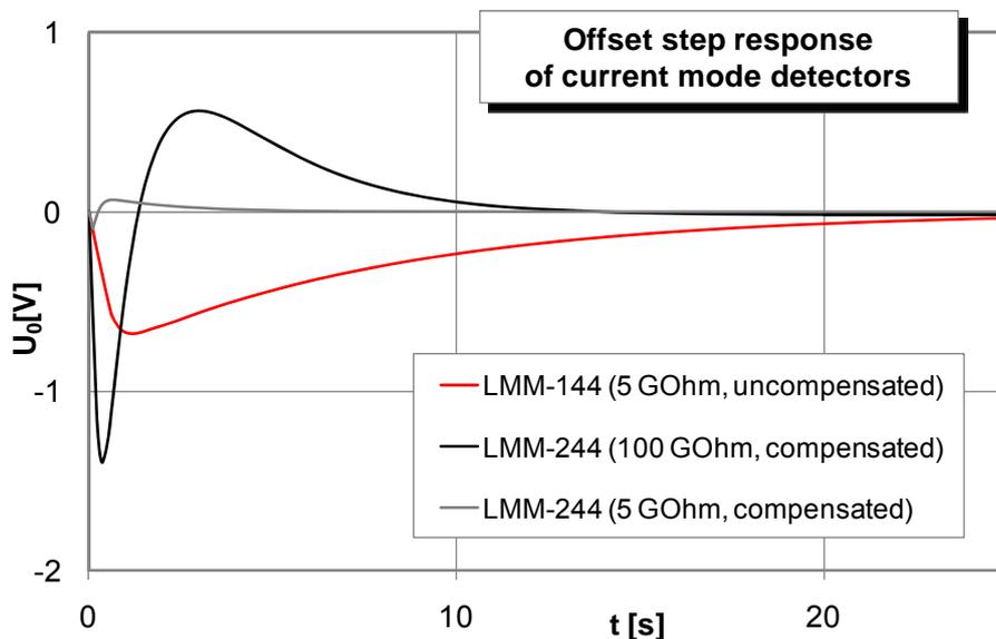
Fig 17: Change of offset voltage vs time of typical current mode detectors after fast temperature increase
