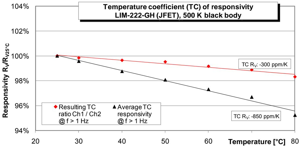
Fig 7: Dual channel detector LIM-222-GH (TO39 housing; small chip size; thermal compensation; JFET; voltage mode; ch1: NBP 3.40  $\mu\text{m}/120\text{ nm HC}$ ; ch2: NBP 3.95  $\mu\text{m}/90\text{ nm Ref.}$ )
