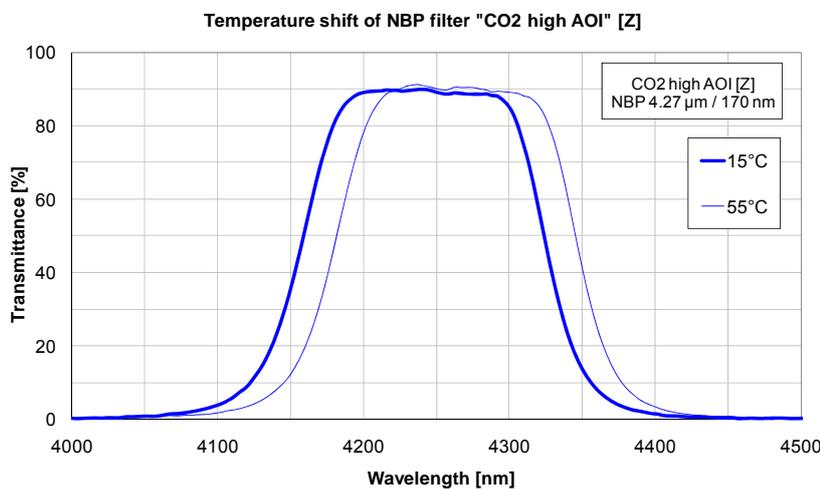
Fig 4: Temperature shift of NBP filter with low angular shift design
