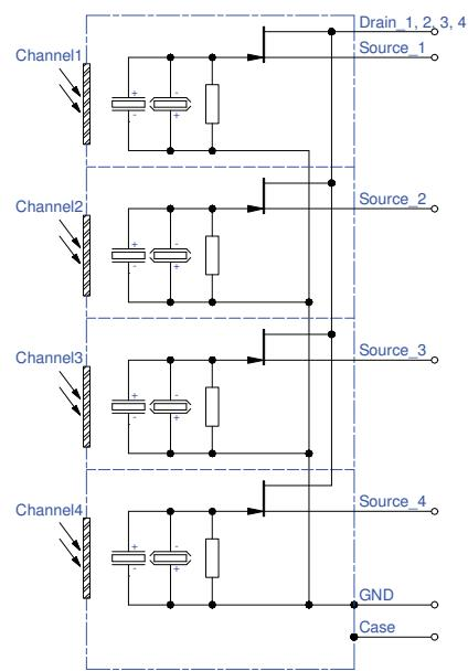
Maximum current between Case and the "Case"-Pin 10 mA!
