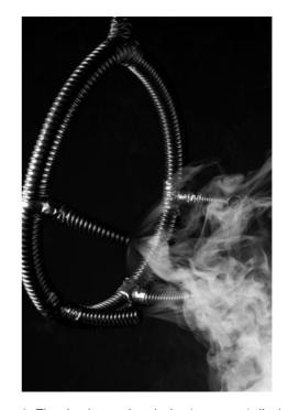
**Figure 1.** The circular suction device (prototype) displaying its efficacy to absorb plume in an experimental setting using a powerful nebulizer with excessive smoke production at low velocity.
