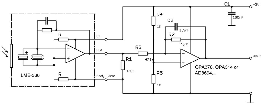
Fig 19: Circuit for current mode (typical  $R_v$  90,000 V/W) of the pyroelectric detector LME-336 (2.7 ... 10) V
