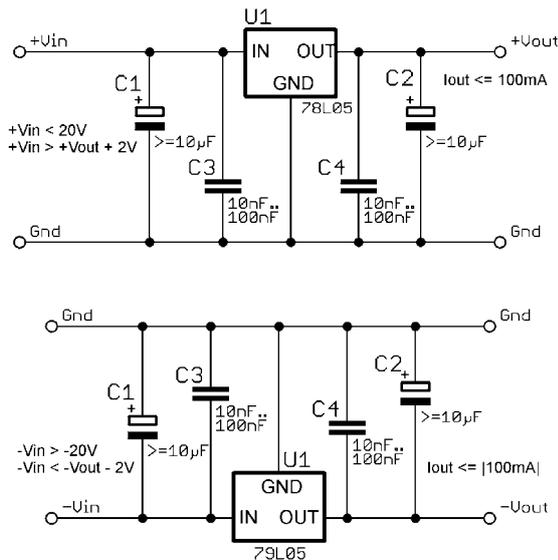
Fig 25: L78L05 fixed +5 V and L79L05 fixed -5 V
