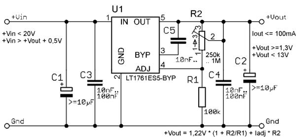
Fig 27: Variable power supply LT1761ES5-BYP for positive voltage
