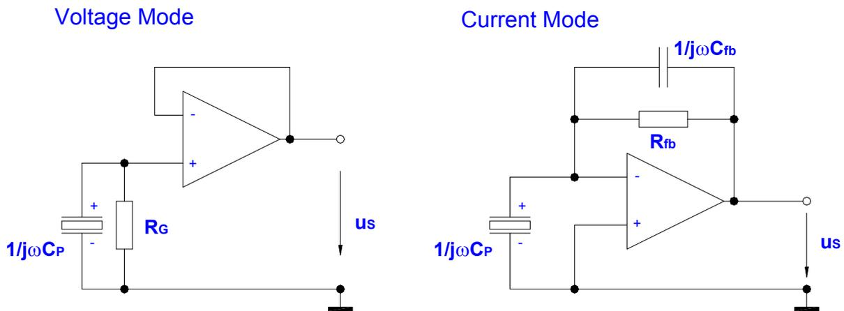
Fig 5: Alternative preamplifier circuits
