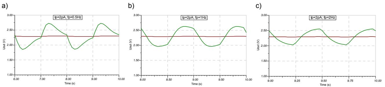
Fig 12:  $U_{out}$  of detector and preamplifier as per figure 10 at different frequencies
