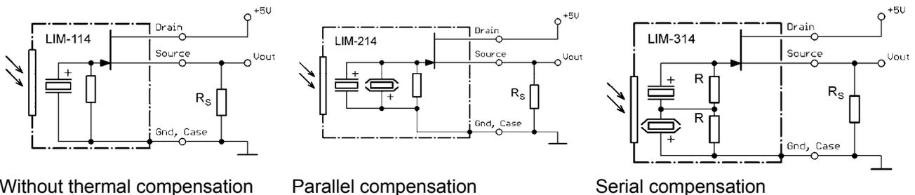
Fig 8: Basic circuits for the voltage mode
