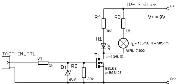
Fig 23: Example: Source MIRL17-900 (Intex) with constant voltage driver
