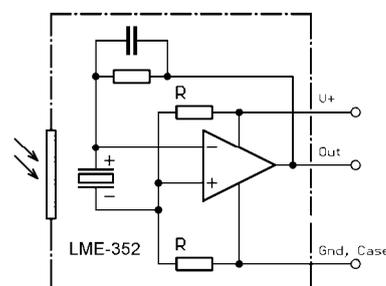
Fig 16: Four alternative pyroelectric detectors suitable for current mode
