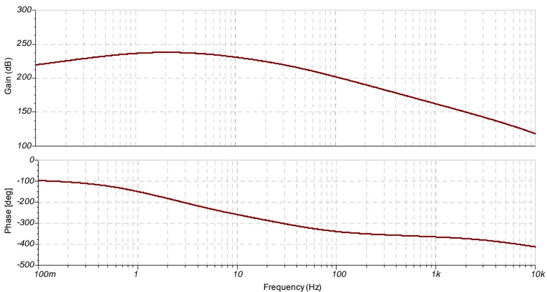
Fig 22: Gain and phase of preamplifier as per figure 21 vs. frequency
