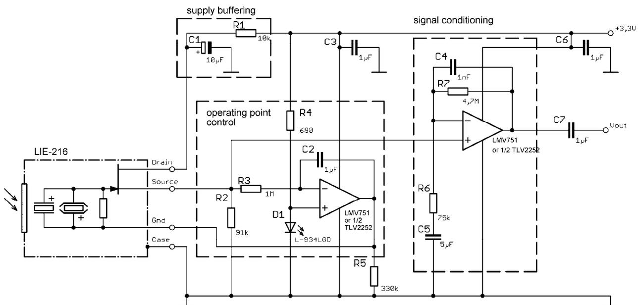
Fig 10: Using TO18 detectors with electrically isolated housing (3.3 V Lithium battery supply; (0.4 ... 33) Hz; gain 60 dB)
