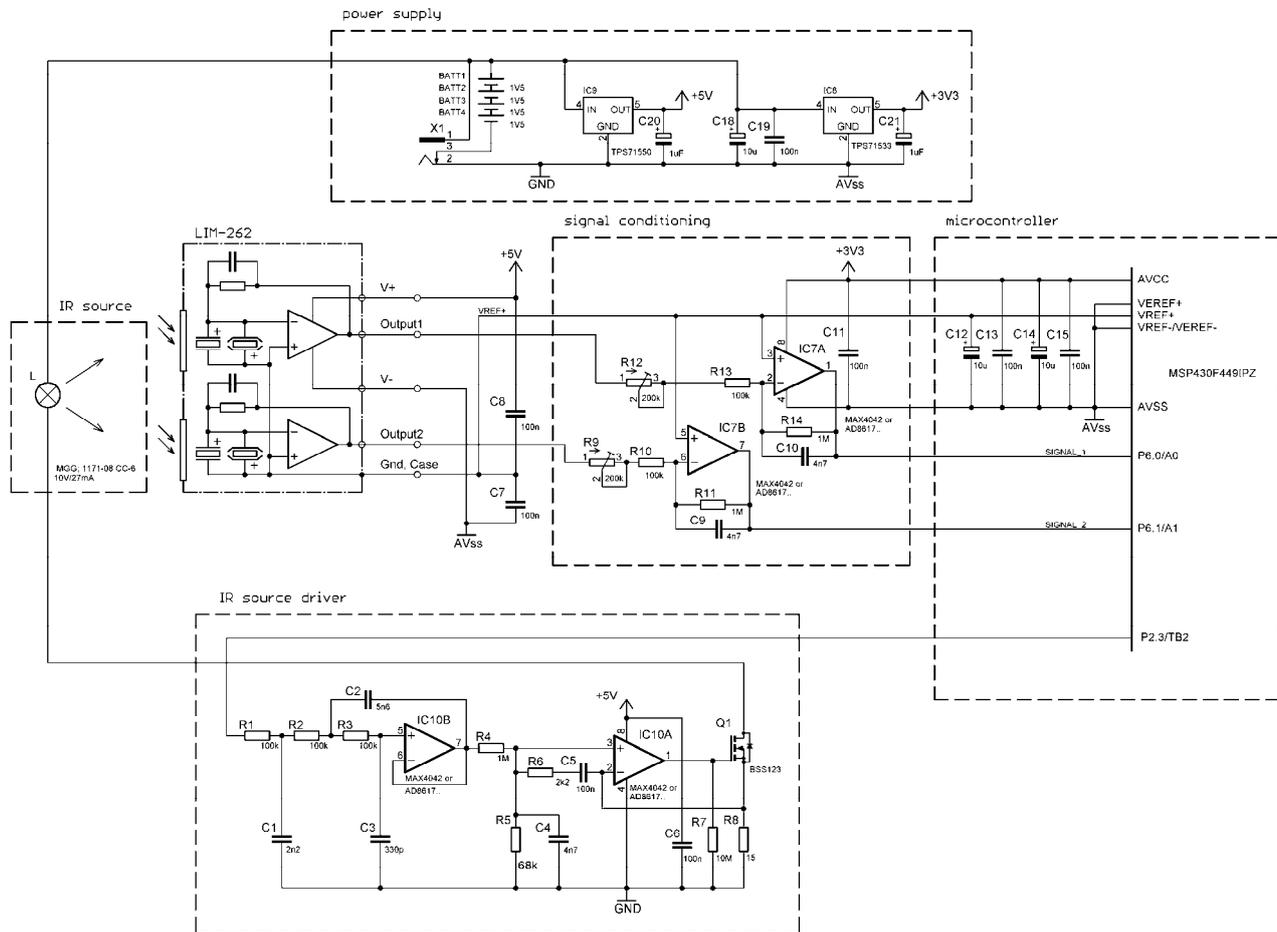
Fig 21: Circuit for current mode of the pyroelectric detectors LIM-262 (typical  $R_v$  60,000 V/W)
