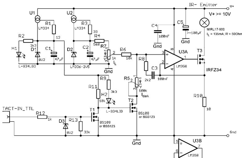
Fig 24: Example: Source MIRL17-900 (Intex) with constant current driver
