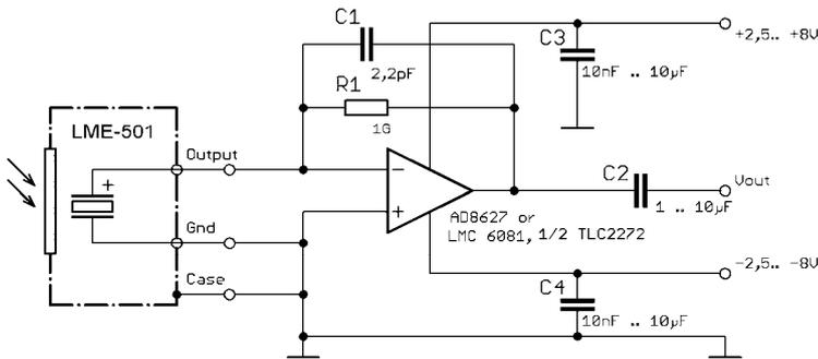
Fig 17: Circuit for current mode ((0.2 ... 25) Hz; 1 V/nA) of the pyroelectric detectors and LME-501
