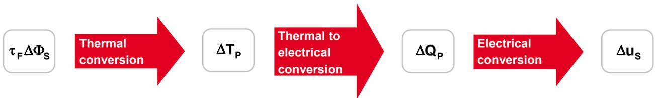
Fig 1: Conversion stages of the pyroelectric infrared detectors
