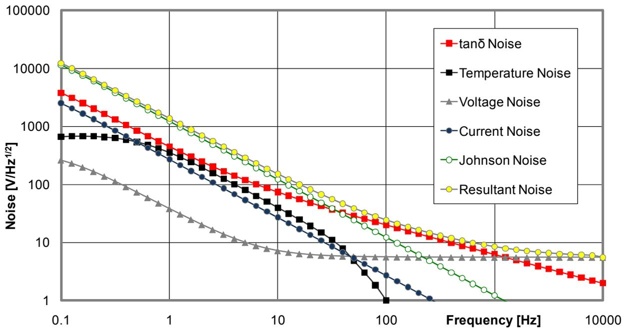
Fig 7: Frequency response of the resulting voltage noise density and of the various components of the voltage noise density of a typical pyroelectric detector (LME-302)
