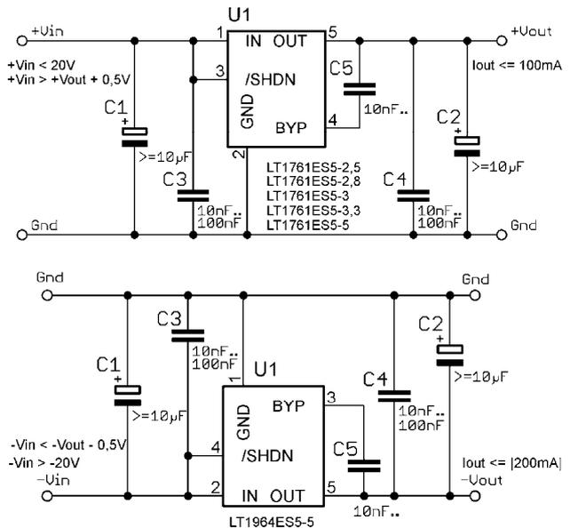
Fig 26: LT1761ES5-X (X=fixed voltage) and LT1964ES5-5 fixed (-5.0 V)
