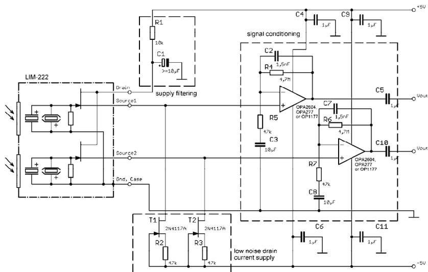
Fig 13: Using dual channel detectors. ( $\pm 5$  V or higher; (0.3 ... 22) Hz; gain 101 dB)
