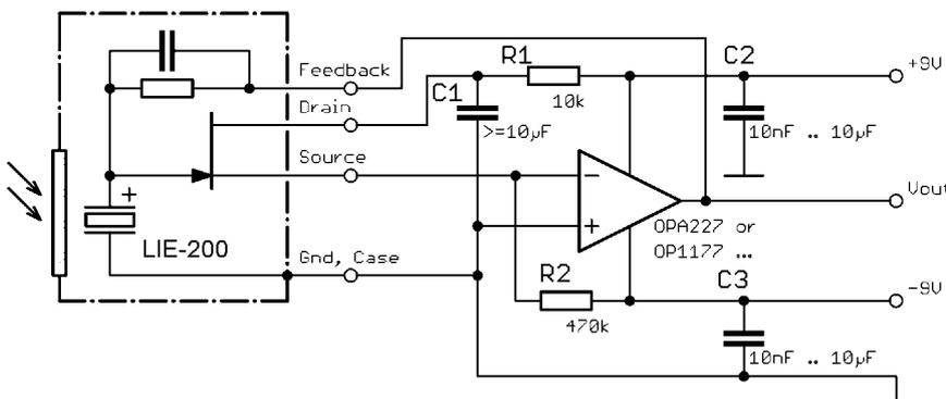
Fig 18: Circuit for current mode of the pyroelectric detector LIE-200
