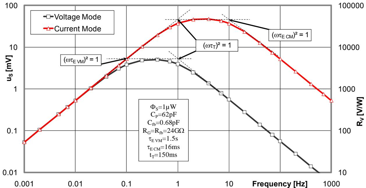
Fig 6: Comparison of the frequency dependencies of signal voltage/responsivity for voltage and current mode
