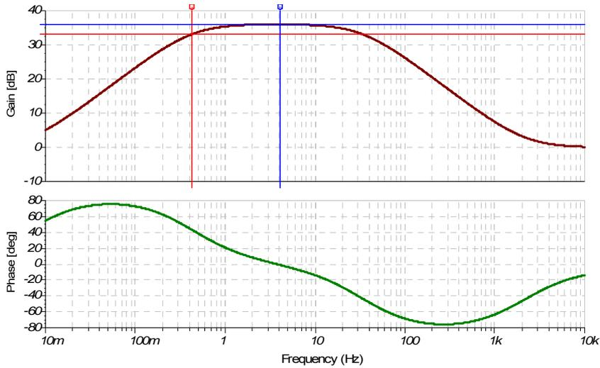
Fig 11: Gain and phase of preamplifier as per figure 10 vs. frequency
