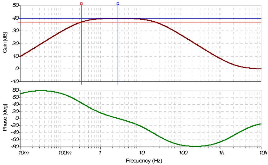
Fig 14: Gain and phase of preamplifier as per figure 13 vs. frequency
