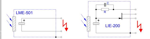
This internal charge and an additional static discharge by unsuitable handling can destroy the detector and/or other electronic devices of the circuitry.
