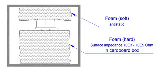
The reason such precautions are taken is that an open circuit pyroelectric chip can generate a voltage of 600 V from a temperature change of 50 °C. This is particularly true of detectors designed to operate in the current mode. Current mode detectors can produce high voltages between pins:
