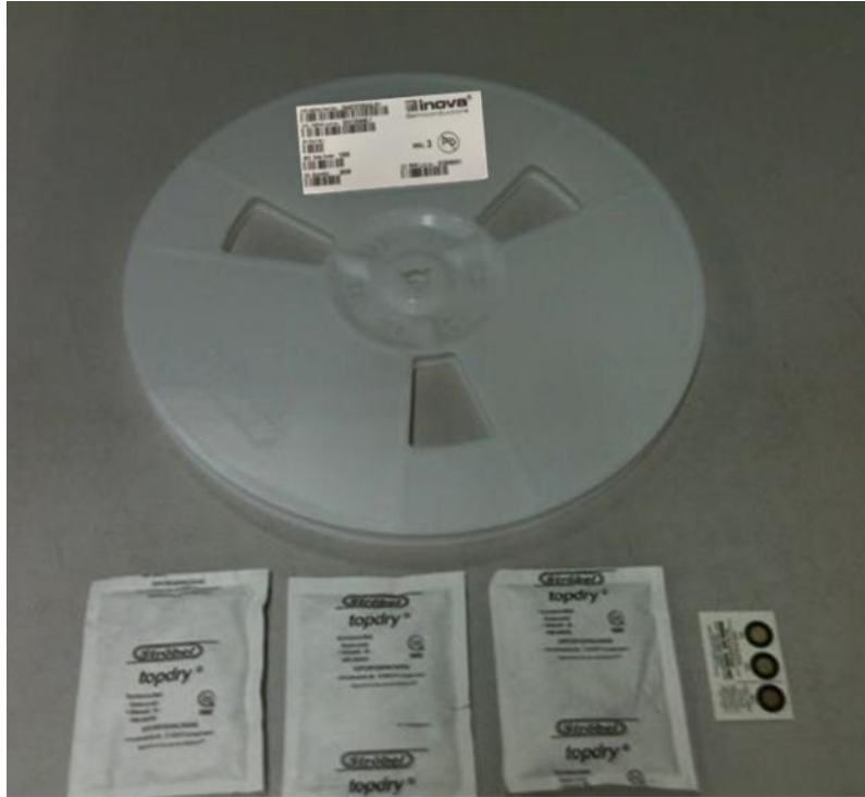
Figure 12 Contents of dry bag for reel
