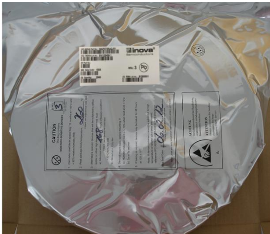
Figure 11 ESD protective dry bag of reel
