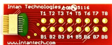
Figure 1. Stim SPI cable adapter board
