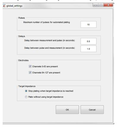
**Maximum number of pulses for automated plating** is described in the automatic plating section. It is often a good idea to set this to a relatively low number (e.g., 2), and run through all electrodes on a new, unplated probe. Any electrodes that can plate quickly will, and any that don't plate will be skipped much more rapidly than if a larger number is used. After the initial quick pass, a larger value may be called for to plate stubborn electrode sites.
