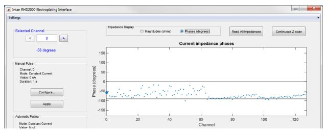
In Phase mode, the phases of the impedances are shown. Again, the selected channel is highlighted. Phases are shown in degrees. Two horizontal black lines indicate phases of 0° (i.e., the impedance is purely resistive) and -90° (i.e., the impedance is purely capacitive).
