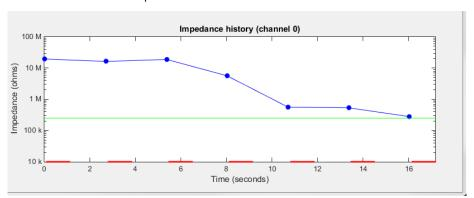
In this plot the plating pulses are shown in red, the measured impedances are shown in blue, and the target impedance is shown in green.
