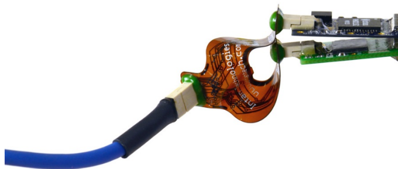
Figure 22. A 96-channel headstage with accelerometer created by combining an RHD2164 amplifier board with an RHD2132 amplifier/accelerometer board.
