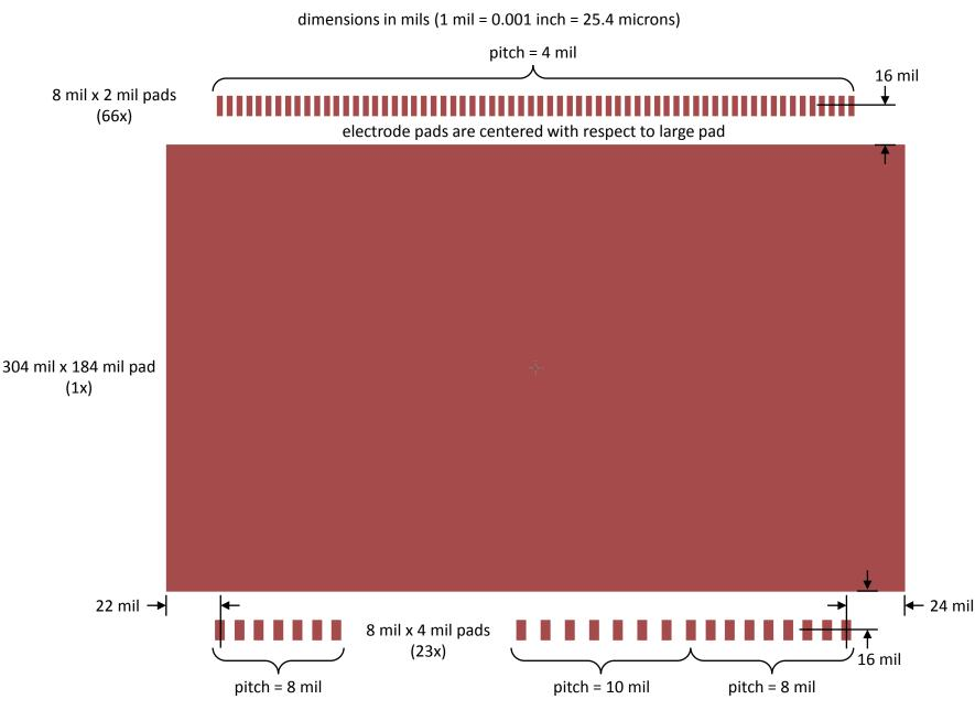
Immersion gold finish (ENIG) or similar planar, bondable finish should be used on PCB.
