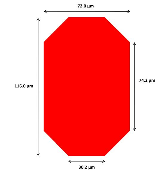
Minimum bond pad pitch (center to center) on RHD2164: 101.6 µm (4.000 mil)
