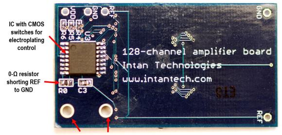
0.06" (1.52 mm) mounting holes (6 mm spacing)
