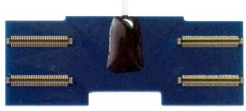
The photo above shows a 256 channel UCLA silicon microprobe. Two RHD2000 128 Channel Amplifier Boards may be connected to this probe (one on either side) to fully instrument all 256 recording sites.
