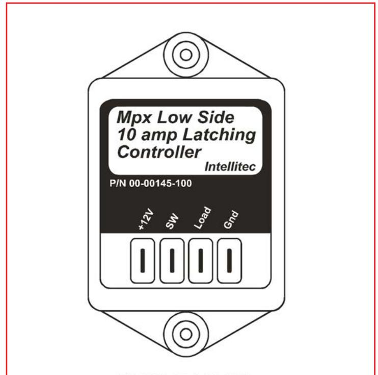
The MONOPLEX™ Water Pump Controller is designed to operate as a “low side”, remote switch in 12 volt DC systems. As it's name implies, it was designed to control the domestic water pump. It's use, however, is not limited to that. It can also be used to control a variety of other loads such as lighting, other pumps, fans, etc., when it is convenient to switch the ground side.
