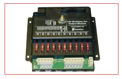
B3=D5. When momentary button D5 is pressed and released output B3 will turn on at 100% intensity and remain on even though switch channel D5 is off. When D5 is pressed and released a second time, output B3 will turn off.
