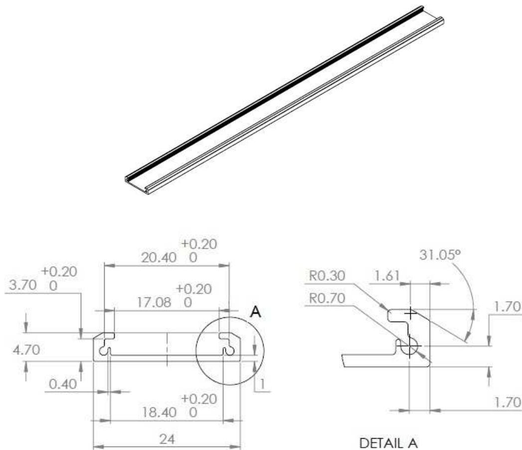
Figure 13: Aluminum extrusion slider architecture
