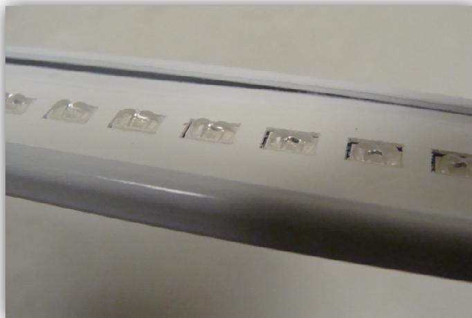
Figure 7: Reflector LED apertures
