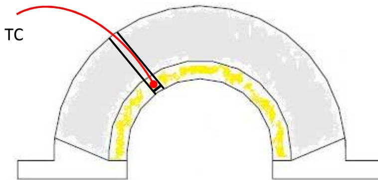
Figure 19: ChromaLit Linear thermocouple insertion
