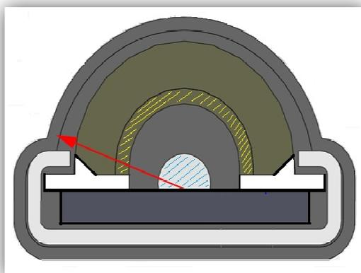
Figure 4: Insertion depth of LEDs
