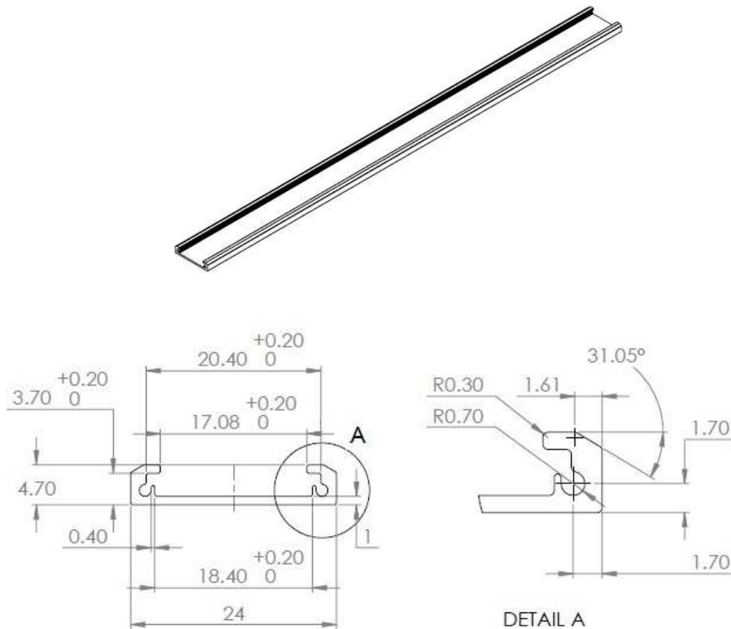
Figure 13: Aluminum extrusion slider architecture
