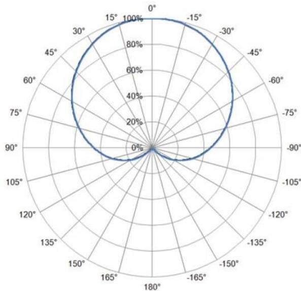
Figure 11: Typical beam angle for standard LIN01 extrusion
