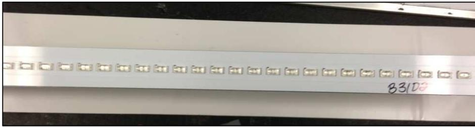
Figure 5: Thermal interface material used under LED PCB
