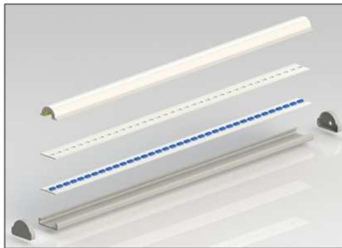
Figure 8: Slider assembly architecture
