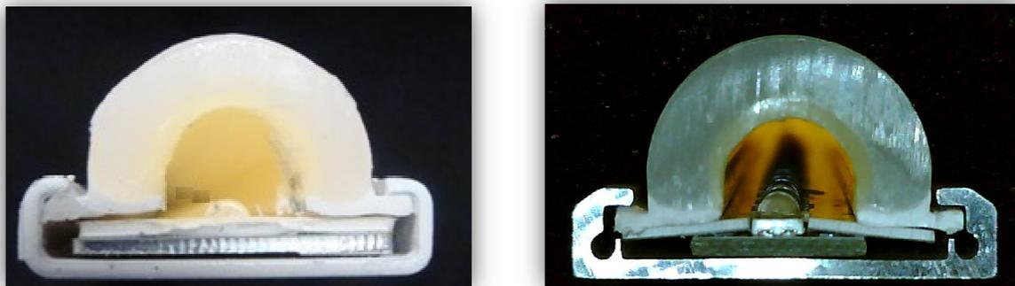
Figure 3: Remote phosphor extrusion in bent aluminum slider assembly (left) and extruded aluminum slider assembly (right); note PCB width is 18mm in left assembly and 10mm wide in right assembly
