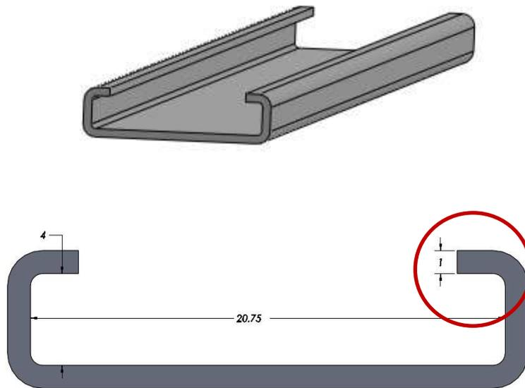
Figure 12: Bent metal slider architecture
