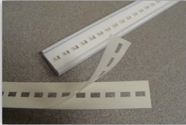
Figure 6: Adhesive backed reflective material
