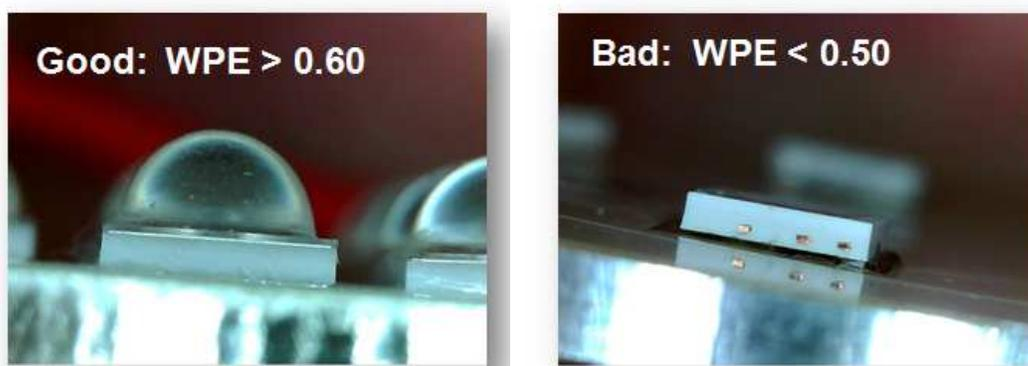
Figure 1: Examples of LEDs with (left) and without (right) extraction surfaces
