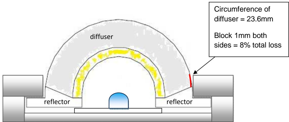
Figure 9: Housing light loss example
