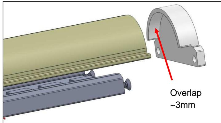
Figure 10: Example of screw on end cap with overlap
