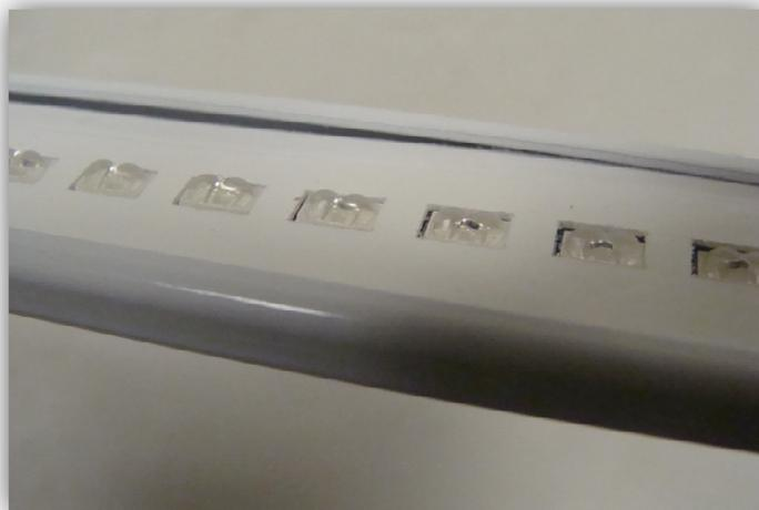
Figure 7: Reflector LED apertures
