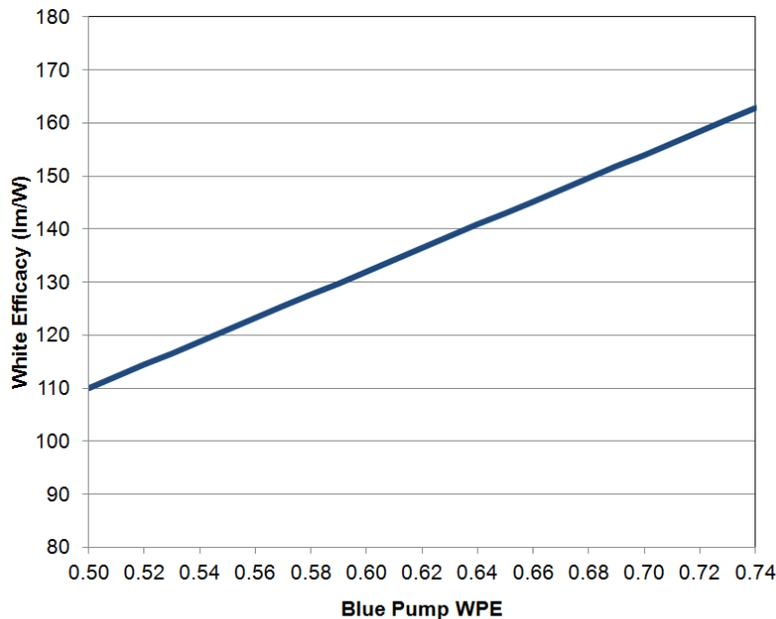
Figure 18: Relationship between white lm/W and WPE for a 220 CE component
