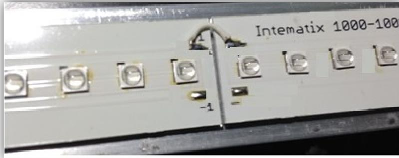
Figure 17: PCB Wiring connection of multiple boards
