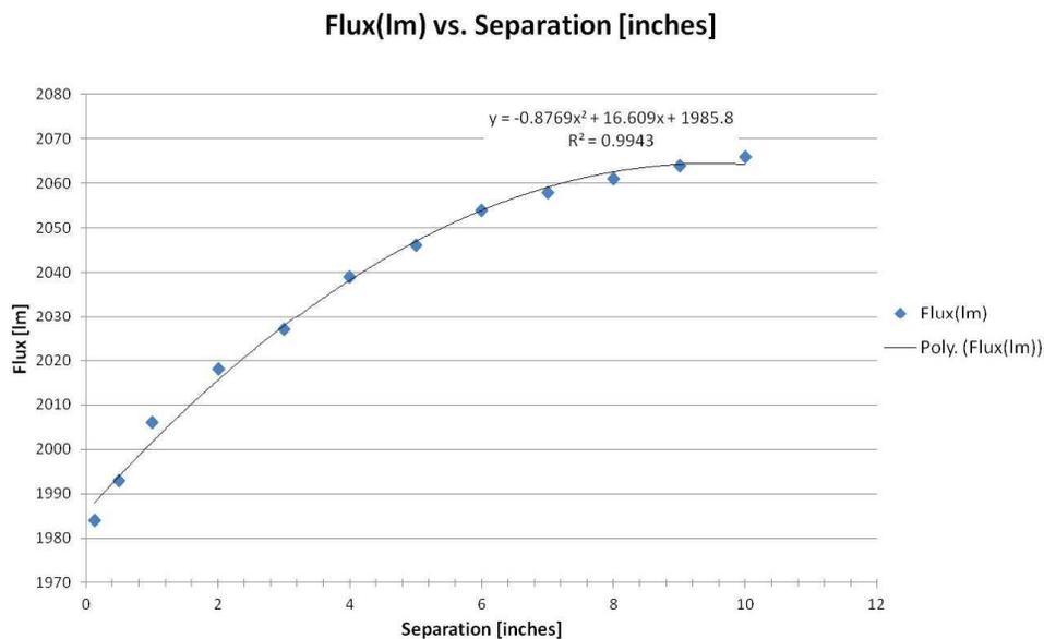
Figure 15: Light loss as a function of center to center spacing of multiple ChromaLit Linear light sources
