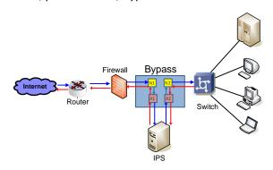
Figure 3: Network Bypass Connected to IPS
