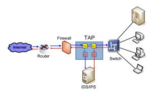
Figure 2: Network TAP Connected to IDS
