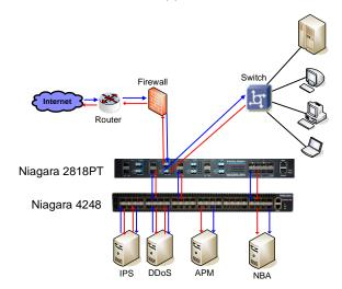
Figure 4: Bypass and NPB
