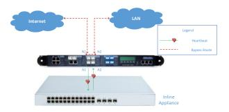
Figure 2: Bypass Mode
