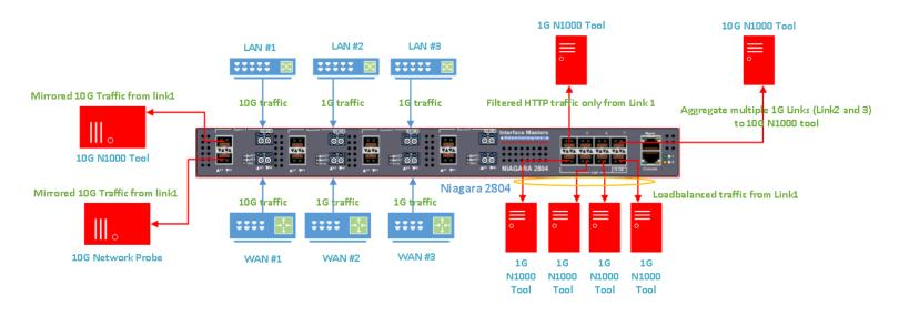
Application Diagram – Interface Masters Niagara 2804 and Reversing Labs N1000 Appliance
