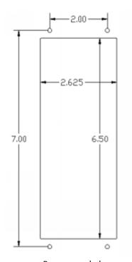
Recommended mounting holes: tap for 8-32 screws
