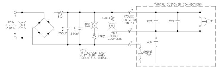
**Note:** Breakers with electronic trip circuits (instead of simple coils) vary widely. Because of this, it is necessary to thoroughly test the 518432/breaker combination to make sure the breaker trips and closes properly.
