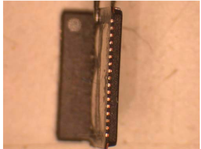
FIGURE 17. FINISHED TINNED THERMAL LAND ON QFN
