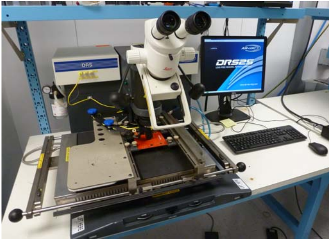
FIGURE 8. REWORK STATION WITH THERMAL PROFILE CONTROL
