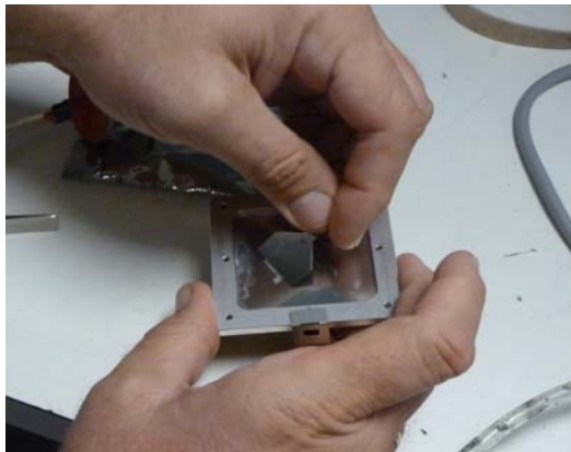
FIGURE 17. DEPOSIT PASTE WITH SMALL SQUEEGEE BLADE
