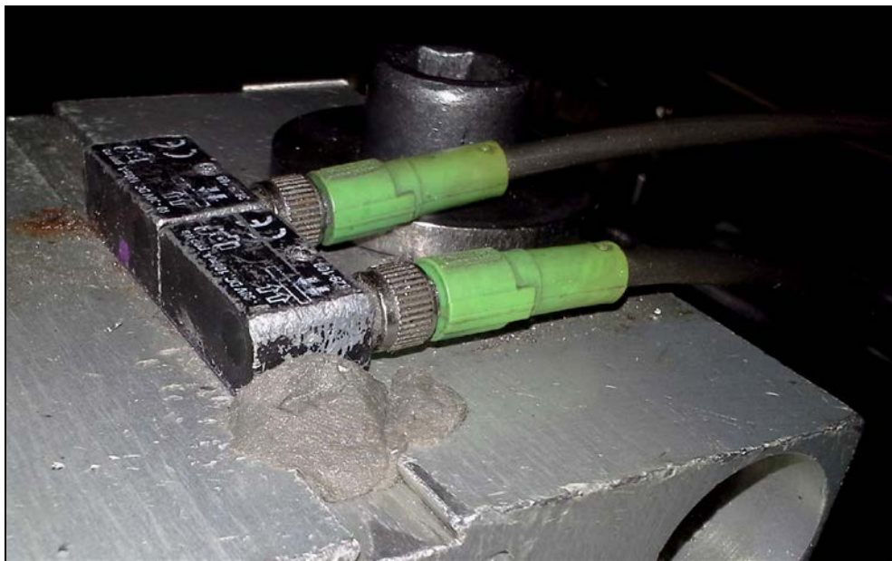
Fig. 5: Magnetic cylinder sensors on a special hydraulic cylinder. The sensors must withstand very high mechanical loads and temperatures of up to +100°C.
