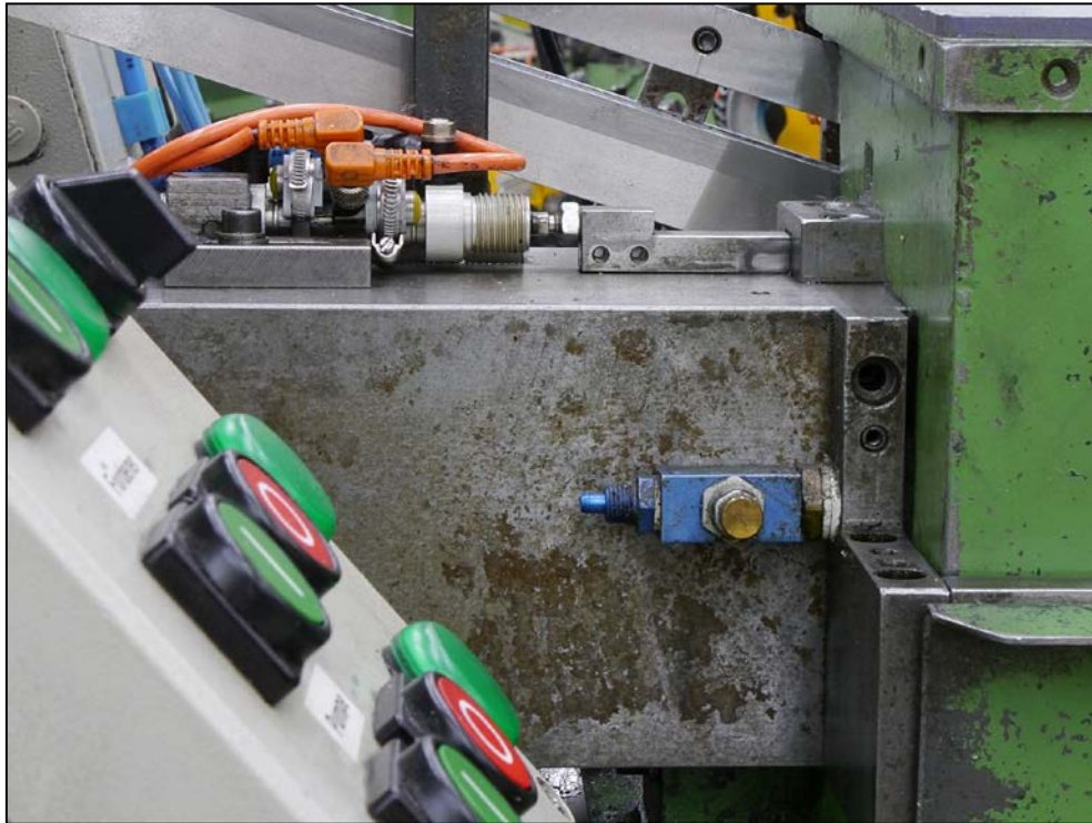
Fig. 6: Two very compact sensors on an extremely short pneumatic cylinder.
