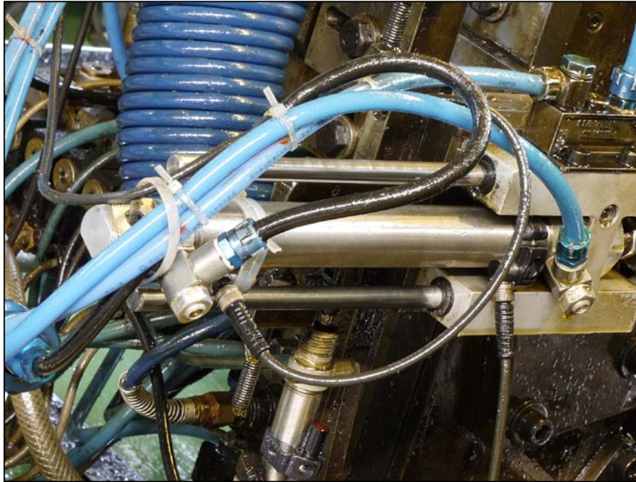
Fig. 8: Cylinder sensors in an extremely oily environment on a machine.
