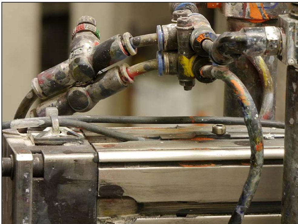
Fig. 7: The sensors even withstand paint splatters, dried-on paint residues or cleaning agents and solvents.
