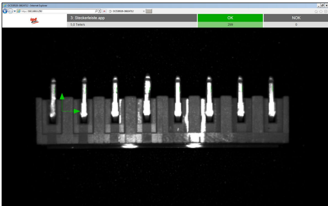
Fig. 8: Features such as a web interface offer various possibilities upon entry of the IP address of the sensor in a standard web browser, such as here for the simple display of test images. Thus, the camera software does not need to be installed on a PC, laptop or tablet for this purpose.
