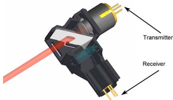
Fig. 6: In the case of devices with coaxial optics, the transmitted and received light beam are on one axis.
