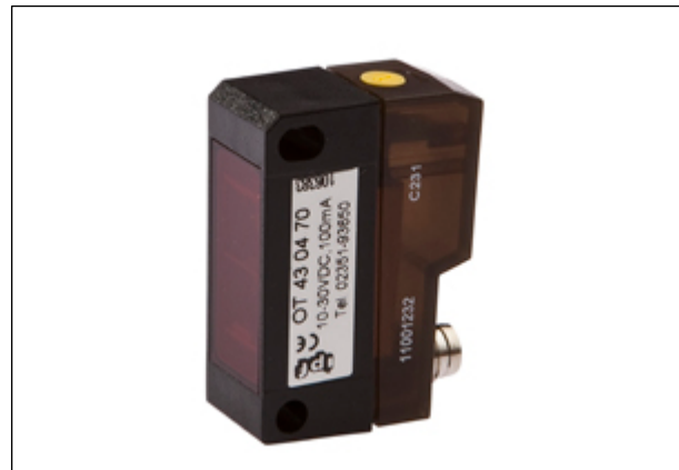
Fig. 10: Diffuse reflection sensors like the OT43 detect material irrespective of color, size and surface.
