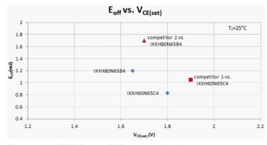
These 650V XPT™ Trench IGBTs are optimized to achieve low switching and conduction losses while maintaining low on-state voltages. The graph demonstrates a superior trade-off (turn-off energy loss vs. on-state voltage) of the new IGBTs (in particular, the IXXH60N65C4 against competitor 1 and IXXH80N65B4 against competitor 2).
