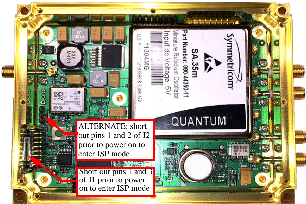
Figure 4.1 Location of header J2 internally to the enclosure
