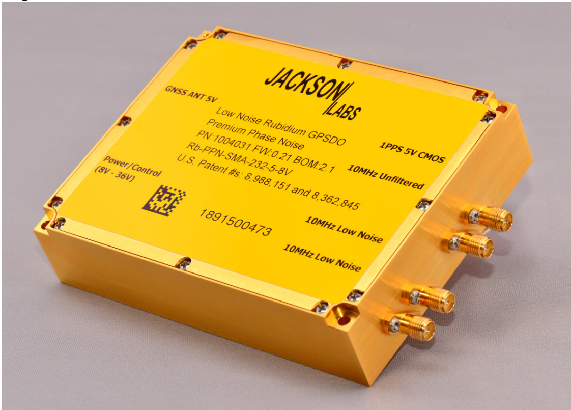
Figure 1.1 Low Noise Rubidium GNSDO
