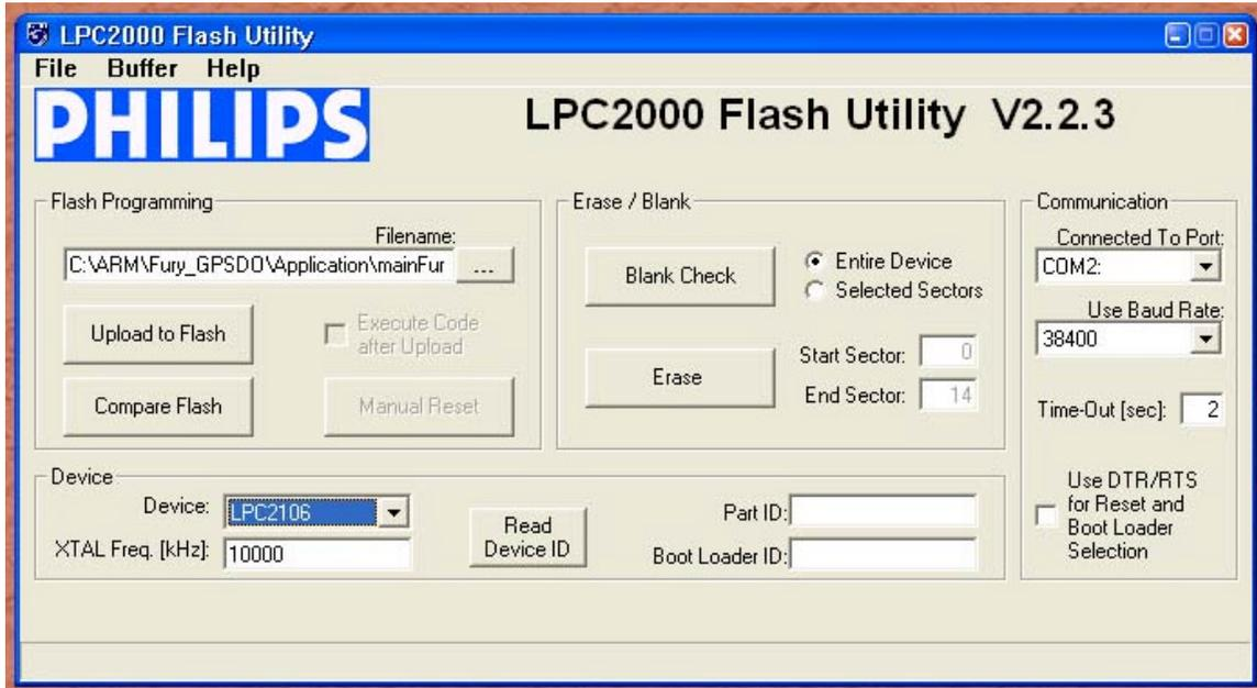
**Please note that the “Use Baud Rate” setting needs to be set to 38400 Baud or less, it will not work faster than 38400 Baud.**
