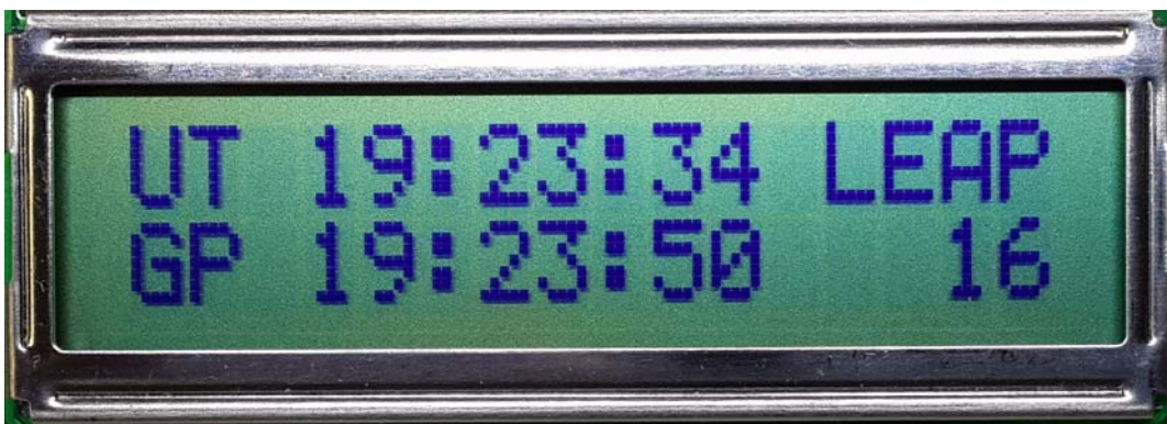
Figure 2.11 GPS/UTC Time display page
