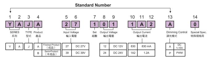
DC to DC LED Driver Part Number ( DC to DC LED 驅動器編碼原則 )
