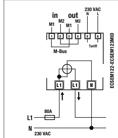
A fuse of 80 A is recommended for the line protection.
