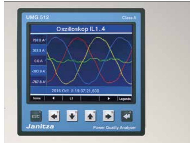
Image 11: Non-linear loads lead to harmonics and return feeding. The measurement shows how these add up on the neutral conductor (green).
