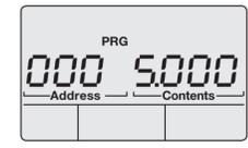
*Fig. Example "Programming mode" display. Address 000 with a contents of 5,000.*
