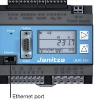
**Fig. Example connection: direct connection between UMG 604/605 and PC. Both devices require a fixed IP address.**
