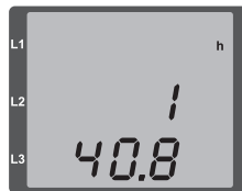
Fig. Measured value indications Operating hours meter
