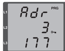
Fig. TCP / IP address, byte 3, value 177
