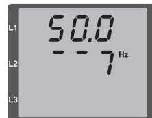
Fig. Indication of the supply frequency (50.0) and the phase sequence.
