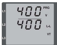
Fig. Programming mode Voltage transformer The primary and secondary currents can be changed using buttons 1 and 2 (cf. page 37).
