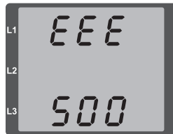
Fig. Warning message with number 500 (mains frequency)
