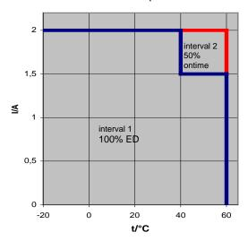
For the duration of on-time only the charge and discharge cycles are relevant. If the buffer-module is charged and works in the standby-modus there is no heating of the unit. From the thermal point of view this can be compared with a switched-off unit.
