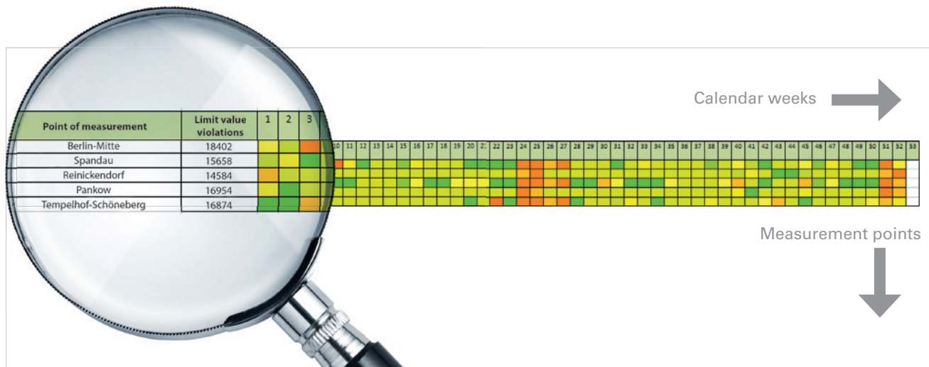
Fig.: Heatmap, i.e. colour (traffic light principle) illustration of how good or bad the power quality was at a particular measurement point in a calendar week. This principle guarantees a quick overview of the complete supply area.
