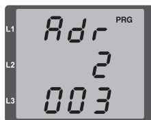
Fig. TCP/IP address Byte 2, value 003
