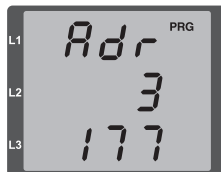
Fig. TCP/IP address Byte 3, value 177
