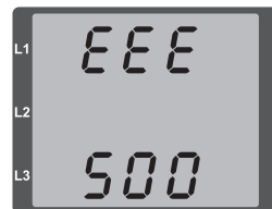
Fig. Warning message with number 500 (mains frequency)
