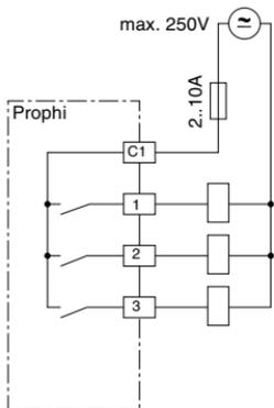
Diagr.: Connection example "Relay outputs"
