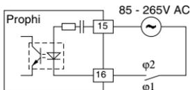
Diagr.: Connection diagram target-cos(phi) changeover
