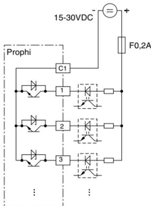
Diagr.: Connection example "Transistor outputs"
