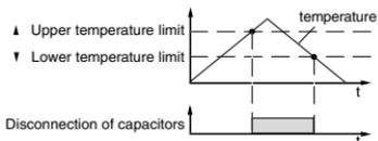
Diagr.: Overtemperature disconnection with hysteresis
