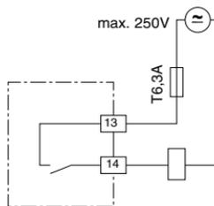
Diagr.: Connection diagram alarm output
