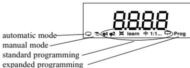
In standard programming often needed settings are carried out such as current transformer ratio or the number of stages.
